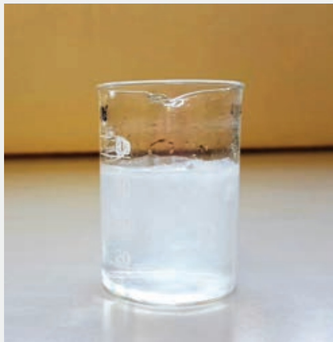
▲ White colour change when an oil adjuvant is added to water.
